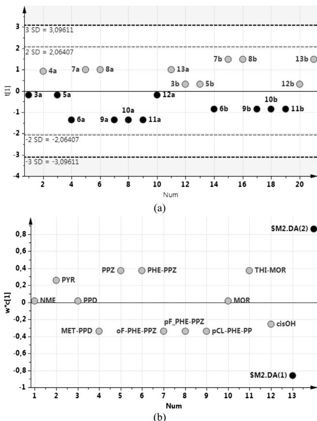
**Fig. 2.** The score plot (a). The first PC accounts for 79% of the variance in the dataset. The highly active compounds with  $MIC < 10 \mu M$  (class 1) are given as black circles. The low active compounds with  $MIC > 10 \mu M$  (class 2) are given as grey circles. The loading plot (b). X and Y descriptors are given as grey and black circles, respectively.
