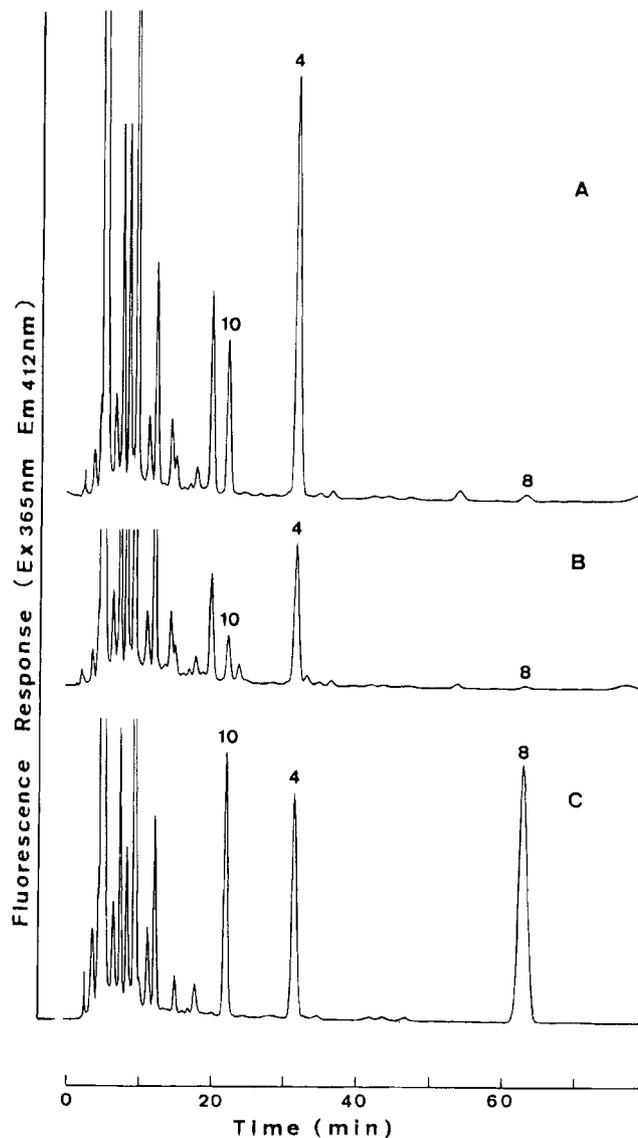
**Figure 3.** HPLC/FLD chromatograms of the ADAM derivatized  $\text{CH}_2\text{Cl}_2$  extracts: (A) ground water; (B) drainage; (C) chemically synthesized standards.
