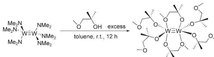
**Scheme 2.** Reaction scheme for the preparation of the bimetallic complex **2**.
