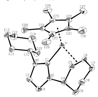
**Figure 2.** PLATON plot of the cation of **4**. All hydrogen atoms are omitted for clarity. Selected bond lengths [Å] and angles [deg]:  $Ir-C_{g1}$  1.895,  $Ir-C_{g2}$  2.044,  $Ir-C_5$  2.145(5),  $Ir-C_6$  2.177(5),  $Ir-C_1$  2.019(4),  $C_5-C_6$  1.400(8);  $C_{g1}-Ir-C_{g2}$  127.09,  $C_{g1}-Ir-C_1$  131.30,  $C_{g2}-Ir-C_1$  87.75,  $C_{g1}-Ir-C_5$  123.23,  $C_1-Ir-C_5$  77.83(17),  $C_5-Ir-C_6$  37.8(2).
