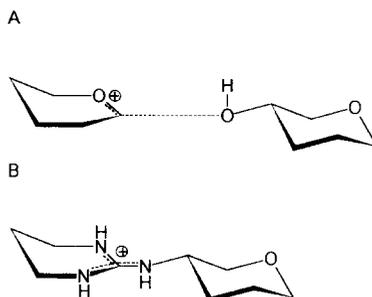
Fig. 2. Hypothetical transition-state of disaccharide heterolysis A in comparison with a disaccharide analogue as transition-state mimic B. In the latter, the cyclic units are pulled together by the guanidinium system, in the former they should drift apart.
