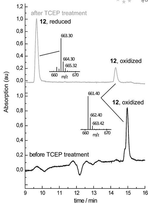
Figure 2. LC-MS traces of isolated auxiliary peptide **12** before and after dissolution in a buffer solution that contained the reducing agent tris(2-carboxyethyl)phosphine (TCEP), which indicates that the oxidized form of the auxiliary peptide is readily reduced under NCL conditions. Absorption was measured at 400 nm.
