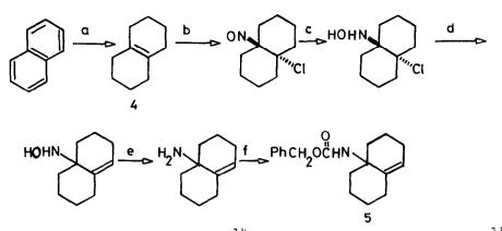
Reagents: (a) Li,  $EtNH_2-Me_2NH^{14}(63\%)$ , (b) <u>iso</u>-amyl nitrite-HCl<sup>15</sup> (70%), (c)  $H_2$ -Pt(98\%)-see Ref 16, (d) NaOMe-MeOH, RT (90%), (e) Al-Hg, THF-H<sub>2</sub>O, reflux (100%)-see Ref 17, (f) PhCH<sub>2</sub>OCOCl (99%).
