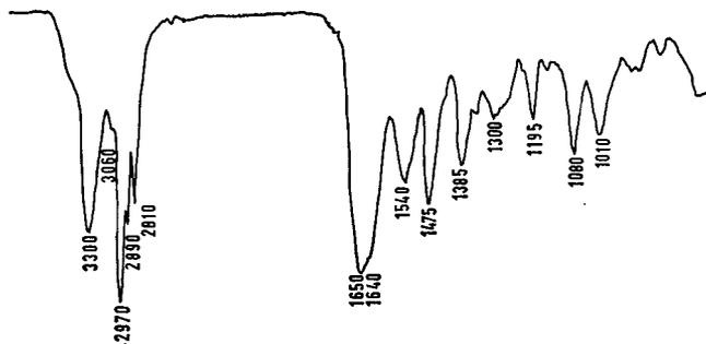
FIG. 2. Infra-red spectrum of  $\delta$ -dipropylaminovalerohydrazide. Liquid film.
