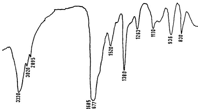
FIG. 1. Infra-red spectrum of formhydrazide, KCl disc.
