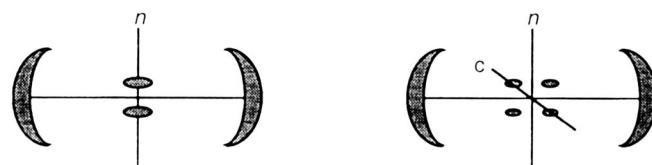
Fig. 1 Schematic representation of the diffraction pattern of a single domain of the nematic phase; the pattern is symmetrical about the director ( n ). Left, usual nematic diffraction pattern; right, nematic with local smectic C ordering as shown by the four spots at small angles (see text)
