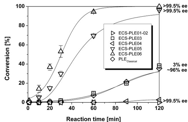
**Figure 2.** Desymmetrization of dimethyl cyclohex-4-ene-*cis*-1,2-dicarboxylate **1** to (1*S*,2*R*)-monoester **2a** depending on the used pig liver esterase isoenzyme. Conditions: 23 °C, 100 mM TRIS buffer pH 7.5, 10 mmol/L substrate; 4 U/mL recombinant PLE (according to the standard activity assay).
