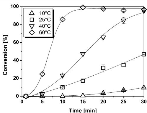
**Figure 3.** Effect of reaction temperature on the ECS-PLE06-catalyzed conversion of dimethyl cyclohex-4-ene-*cis*-1,2-dicarboxylate. Conditions: 50 mM phosphate buffer pH 7.5, 10 mM substrate; 4 U/mL recombinant PLE (according to the standard activity assay).
