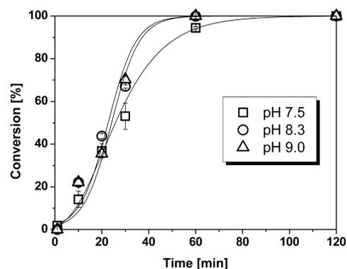
**Figure 4.** Effect of pH on the ECS-PLE06-catalyzed conversion of dimethyl cyclohex-4-ene-*cis*-1,2-dicarboxylate. Conditions: 50 mM phosphate buffer, 23 °C, 10 mM substrate; 4 U/mL enzyme (according to standard activity assay).
