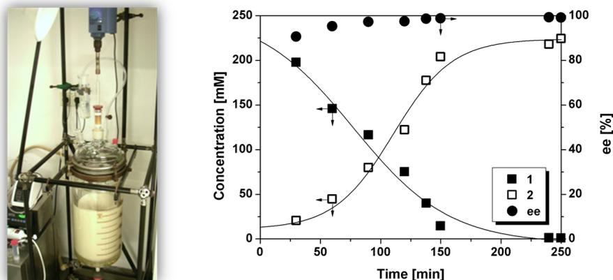
**Figure 6.** Scaled-up desymmetrization of dimethyl cyclohex-4-ene-*cis*-1,2-dicarboxylate. (Left) Temperature-controlled bioreactor with a total capacity of 10 L. (Right) Time course of concentration of reagent **1** (■), concentration of product **2** (□), and ee (●) as determined by GC analysis. Conditions: 200 mM substrate, 5.5 U/mL ECS-PLE06, total volume 8.8 L, stirrer speed 300 rpm, 40 °C, pH control via acid scavenger NaHCO<sub>3</sub>.
