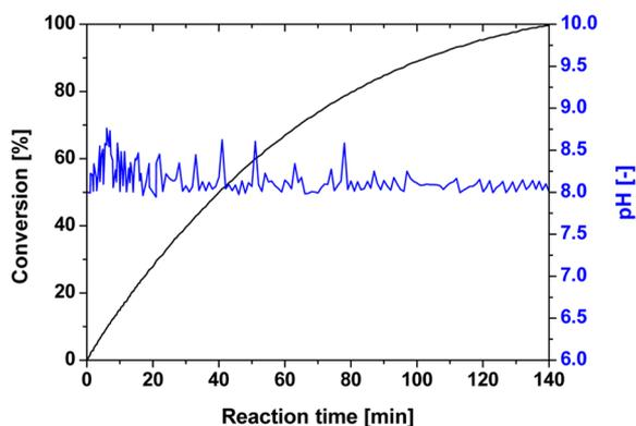
**Figure 5.** pH-dependent addition of a base solution causes fluctuations of the pH, depending on the reactor geometry, especially during the beginning of the reaction. Conditions: total volume 0.04 L, 80 mM substrate, 40 °C, pH control with 0.5 M NaOH solution, pH measurement near the buret; conversion was calculated from NaOH consumption.
