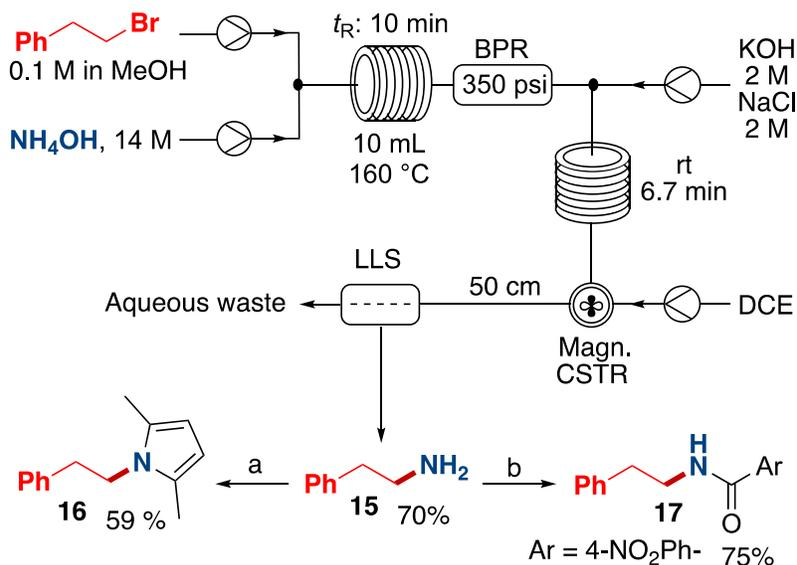
All flow pumps are fixed to 0.5 mL·min<sup>-1</sup>; Magn.CSTR: Magnetic Continuous Stirred Tank Reactor; LLS: Liquid-Liquid Separator; a) Acetylacetone (1.05 equiv), 100 °C, 1 h; b) 4-Nitrobenzoyl chloride (2.4 equiv), NEt<sub>3</sub> (2.4 equiv), 25 °C, 1 h.
