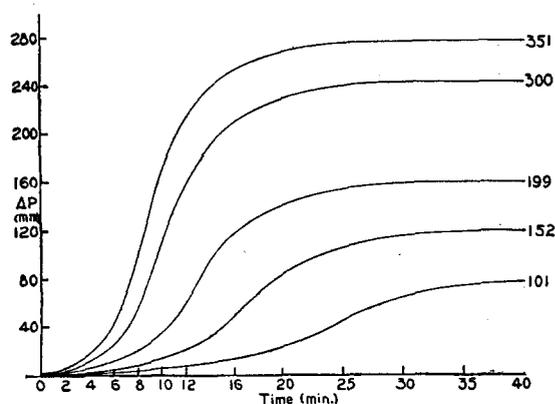
FIG. 2. Decomposition rate curves of propyl mercaptan at pressures of 101, 152, 199, 300 and 351 mm at  $405^{\circ}\text{C}$ .
