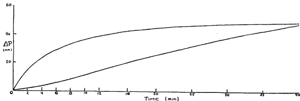
FIG. 5. Decomposition rate curves of propyl sulphide (lower) and propyl sulphide and hydrogen sulphide (upper).
