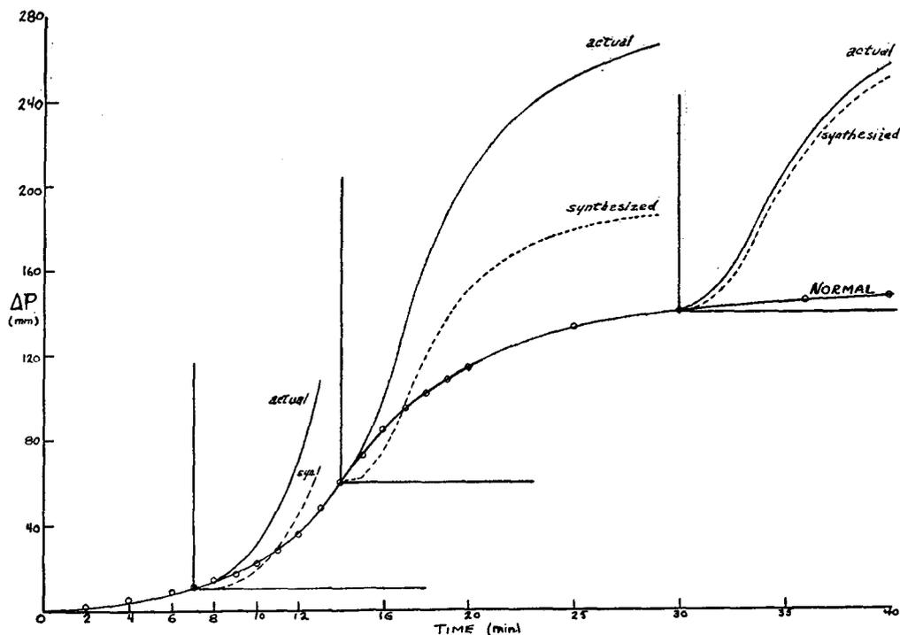
FIG. 4. Composite diagram of the effects of three separate additions of propyl mercaptan to 181 mm already partially decomposed at 405°C. Sample 1 of 172 mm injected after 7 min. Sample 2 of 177 mm injected after 14 min. and sample 3 of 181 mm, after 30 min.
