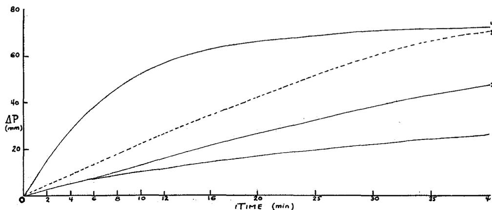
FIG. 6. Rate curves for the decomposition of (1) propyl mercaptan, (2) propyl sulphide, (4) a mixture of both. Curve (3) for comparison is the result of adding the ordinates of (1) and (2).
