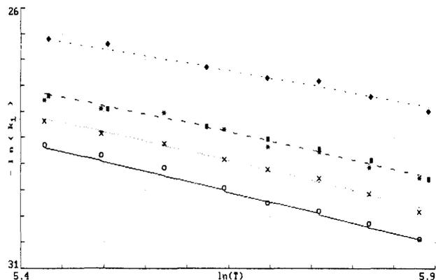
**Figure 4.** Dependence of  $k_1$  on temperature at different pressures of  $N_2$ . Experimental points: (O) this work at 25 Torr; (X) this work at 50 Torr; (\*) this work at 100 Torr; (■) ref 5 at 100 Torr; (▲) ref 5 at 700 Torr. The lines drawn at each pressure come from a fit of this complete data set to eq I-III.
