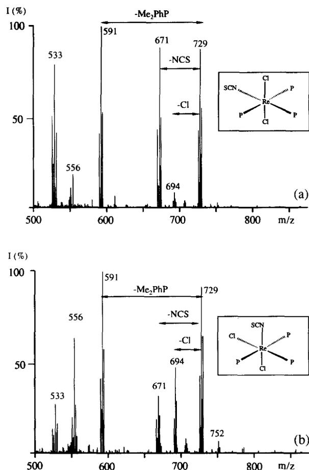
Fig. 3. FAB<sup>+</sup> mass spectra of (a) *trans*- and (b) *cis*-[ReCl<sub>2</sub>(NCS)(Me<sub>2</sub>PhP)<sub>3</sub>] (merged from each 30 individual spectra; matrix: nitrobenzylalcohol).
