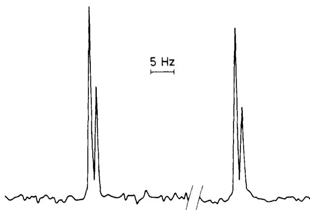
Figure 2. The complete proton-decoupled <sup>77</sup>Se NMR spectrum of the cis and trans dimethyl-diethyl-TSF mixture.
