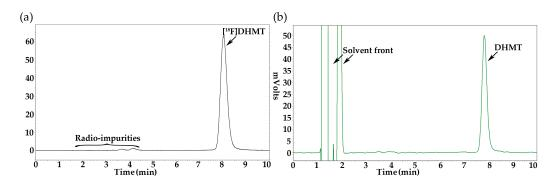
**Figure 2.** Analytical HPLC chromatograms for [<sup>18</sup>F]DHMT: (**a**) radioactivity detection; (**b**) UV, with co-injection of [<sup>19</sup>F]DHMT.
