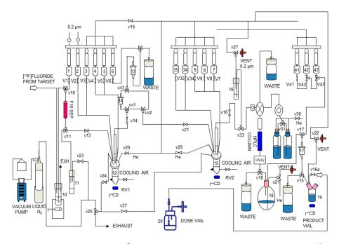
Figure 4. Schematic of the TRACERLab® FXN Pro automated module for radiosynthesis of [18F]DHMT.
