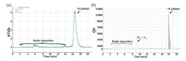
**Figure 1.** Semi-preparative radio-HPLC chromatograms for purification of [<sup>18</sup>F]DHMT ([<sup>18</sup>F]5). (a) Manual method; (b) Automated method.
