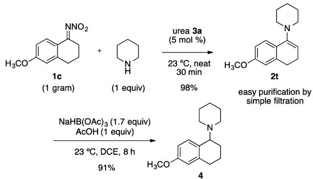
As demonstrated in the formation of enamines **2e**, **2f**, and **2g**, the urea-catalyzed cross-coupling of aliphatic amines and nitrimines is highly efficient, producing high yields with few byproducts in solvent-free conditions. We found the reaction to be suitable for the preparation of enamines on a large scale without the need for significant purification (Scheme 5). For example, on a gram scale,
