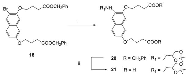
**Scheme 2** Reagents and conditions: (i) (2,2-dimethyl-[1,3]-dioxolan-4-yl)-methylamine, amination reaction. (ii) H<sub>2</sub>, 10% Pd/C, CH<sub>3</sub>OH–EtOAc (1 : 1, v/v), r.t., 24 h.
