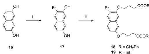
**Scheme 1** Reagents and conditions: (i) Br<sub>2</sub>, CH<sub>3</sub>COOH, 1.5 h, then Sn powder, H<sub>2</sub>O, 80 °C, 24 h. (ii) Br(CH<sub>2</sub>)<sub>3</sub>COOCH<sub>2</sub>Ph or Br(CH<sub>2</sub>)<sub>3</sub>COOEt, K<sub>2</sub>CO<sub>3</sub>, dry DMF, 50 °C, overnight.
