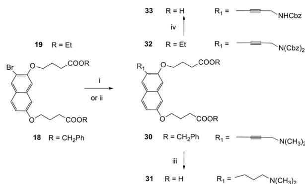
**Scheme 4** Reagents and conditions: (i) **18**, *N,N*-dimethylpropargylamine, CuI (10 mol%), Pd(PPh<sub>3</sub>)<sub>4</sub> (5 mol%), Et<sub>3</sub>N, DMF, 80 °C, 6.5 h. (ii) **19**, *N,N*-di(benzyloxycarbonyl)propargylamine, CuI (10 mol%), Pd(PPh<sub>3</sub>)<sub>4</sub> (5 mol%), Et<sub>3</sub>N, DMF, 80 °C, 15 h. (iii) H<sub>2</sub>, 10% Pd/C CH<sub>3</sub>OH–EtOAc 1 : 1 (v/v), r.t., 14 h. (iv) NaOH<sub>aq</sub> 2 N, CH<sub>3</sub>OH–THF 1 : 1 (v/v), r.t., 5.5 h, then HCl<sub>aq</sub> 1 N.
