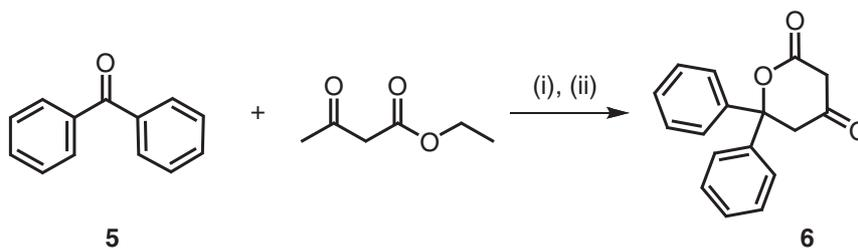
**Scheme 4.** Synthesis of  $\beta$ -keto  $\delta$ -lactone **6**. Reagents and conditions: (i) NaH, *n*-BuLi, THF, 0 °C; (ii) NaOH, THF, 0 °C.
