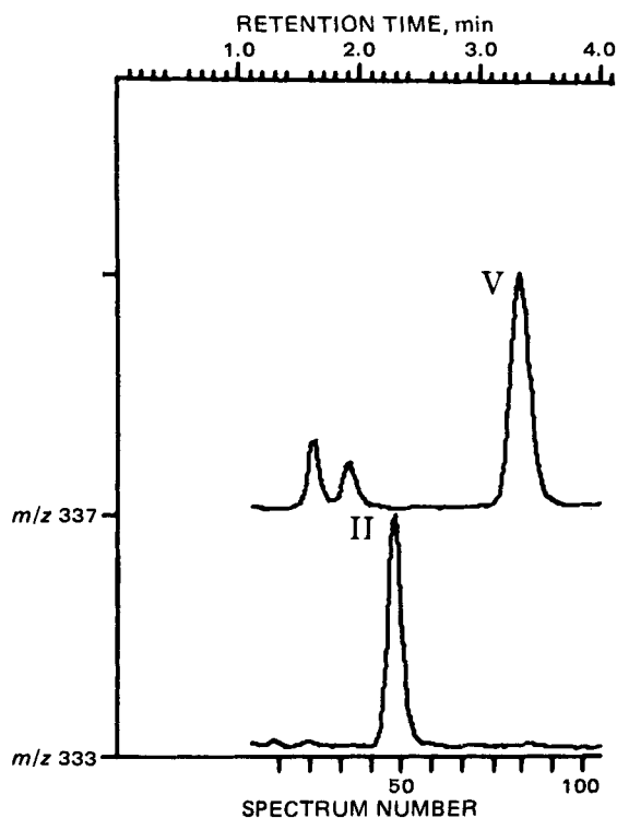
Figure 10 —Selected ion monitoring (chemical-ionization mode) tracing of ethylated human plasma (nonhydrolyzed) extract. For additional details, see Fig. 9.
