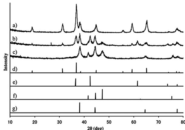
**Fig. 3** XRD patterns of Au/Co<sub>3</sub>O<sub>4</sub>. (a) after air calcination, (b) after H<sub>2</sub> treatment (2 MPa, 100 °C, 3 h, in heptane), (c) after intermolecular hydroaminomethylation reaction (1-hexene and *N*-isopropylaniline, 120 °C, 4 h, CO/H<sub>2</sub> = 1 : 1, 4 MPa, in heptane). The patterns of (d) Co<sub>3</sub>O<sub>4</sub>, (e) CoO, (f) Co, and (g) Au are shown based on JCPDS data.
