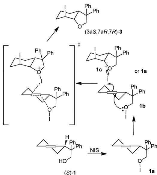
**Scheme 2.** Proposed reaction mechanism of cyclohaloetherification.
