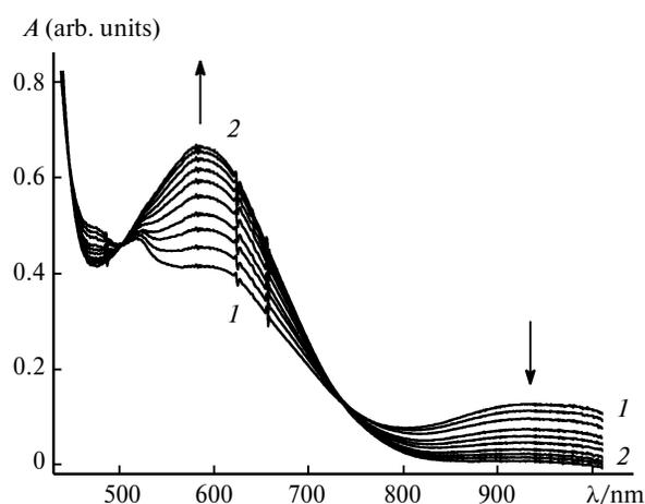
**Fig. 4.** Absorption spectra of complex **2b** in toluene in the temperature range from 283 (**1**) to 328 K (**2**) with an increment of 5 K,  $C_{\mathbf{4b}} = 8.32 \cdot 10^{-5} \text{ mol L}^{-1}$ .
