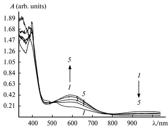
**Fig. 5.** Absorption spectra of complex **2b** in toluene at the constant product  $C_{\mathbf{2b}} \cdot l = 1.22 \cdot 10^{-3} \text{ mol cm L}^{-1}$  at optical path-length  $l = 0.1$  (**1**), 0.5 (**2**), 1.0 (**3**), 2.0 (**4**), and 5.0 cm (**5**),  $T = 293 \text{ K}$ .
