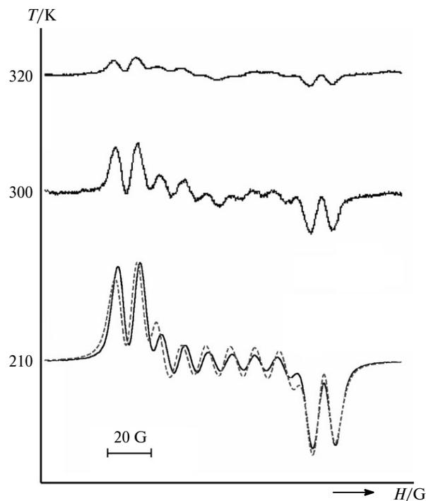
**Fig. 2.** ESR spectra of compound ISQ-**2b** in a toluene solution at different temperatures ( $a^N = 15.4 \text{ G}$ ,  $a^{Co} = 12.0 \text{ G}$ ,  $g = 1.9936$ ) and the simulated ESR spectrum at 210 K (dashes).
