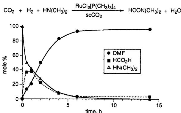
**Figure 1.** The composition of the product as a function of reaction time for the reaction of dimethylammonium dimethylcarbamate (5.0 mmol), H<sub>2</sub> (80 atm), and scCO<sub>2</sub> (130 atm) at 100 °C catalyzed by RuCl<sub>2</sub>[P(CH<sub>3</sub>)<sub>3</sub>]<sub>4</sub> (2.5 μmol) in a 50-mL vessel.
