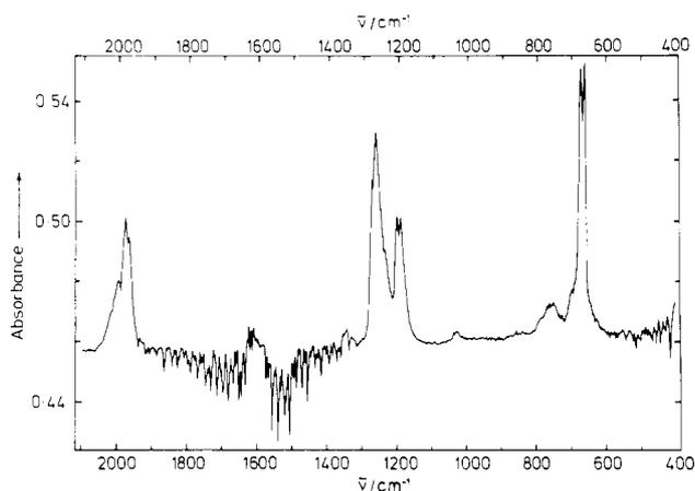
**Figure 1.** FT-IR spectrum of gallane vapor in a Pyrex glass cell with a pathlength of 10 cm, fitted with CsI windows and cooled to ca. 270 K; the record corresponds to the difference in absorbance between the initial, partially decomposed and final, fully decomposed sample (with appropriate scaling).
