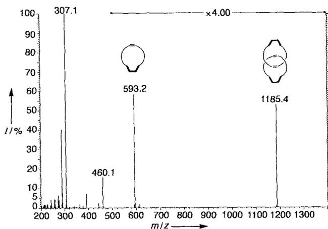
Figure 2. Positive FAB-MS spectrum of catenane **13** in a *p*-nitrobenzyl alcohol matrix (display from  $m/z = 200$  to  $1400$ ; peaks at  $m/z = 307.1$  and  $460.1$  result from the alcohol matrix). The peak at  $m/z = 1185.4$  corresponds to [catenane  $- H^+$ ], and at  $m/z = 593.2$  to [macrocycle  $- H^+$ ]. The absence of peaks between the molecular ion peak and the peak corresponding to the individual macrocycle is characteristic for catenated species [16].
