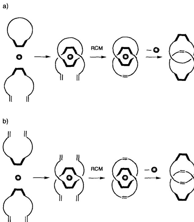
Figure 1. Schematic drawing of the approach utilizing a combination of a transition metal based template strategy and RCM to provide access to [2]catenanes: a) formation of a threaded complex followed by RCM and decomplexation; b) formation of an intertwined complex followed by RCM and decomplexation. The black circle represents the transition metal ion.
