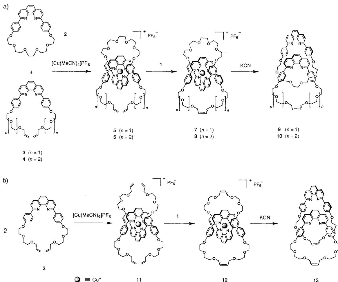
Scheme 1. Synthesis of the [2]catenanes **9**, **10**, and **13**. a) RCM of the threaded complexes **5** and **6** resulting in a 32- and 38-membered ring, respectively. b) RCM of the intertwined complex **11** resulting in two 32-membered rings.
