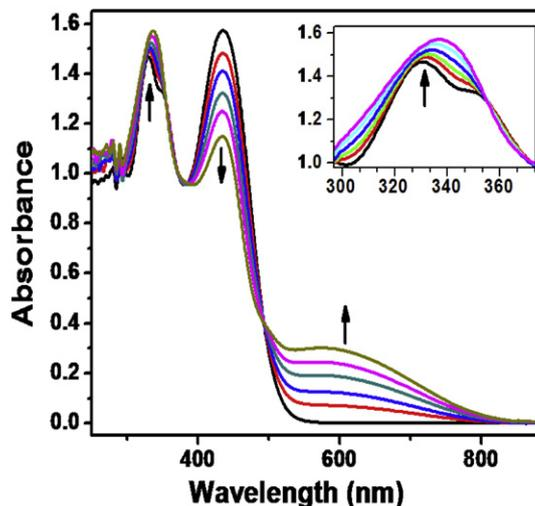
**Fig. 2.** UV-vis spectral changes of **C3** upon titration with TCNE (0–1.0 equiv) in chloroform at 20 °C. Inset: zoom on the low energy CT band.
