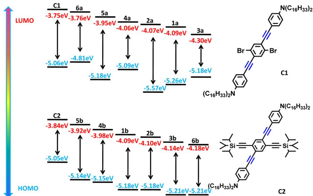
Fig. 3. HOMO and LUMO energy levels of **C1**, **C2** and products **1–6a**, **1–6b**. On the right are the chemical structures of **C1** and **C2**.
