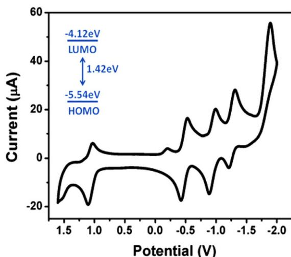
Fig. 4. Cyclic voltammogram of **7a** in  $\text{CH}_2\text{Cl}_2/\text{Bu}_4\text{NPF}_6$  at  $20$  °C. Inset: HOMO and LUMO of product **7a**.
