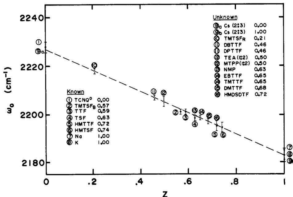
Figure 1. Nitrile stretching frequency,  $\omega_0$ , vs.  $Z$  for 19 TCNQ salts. (●)  $Z$  known from independent measurements;<sup>17,19</sup> (○)  $Z$  previously unknown.<sup>17</sup>
