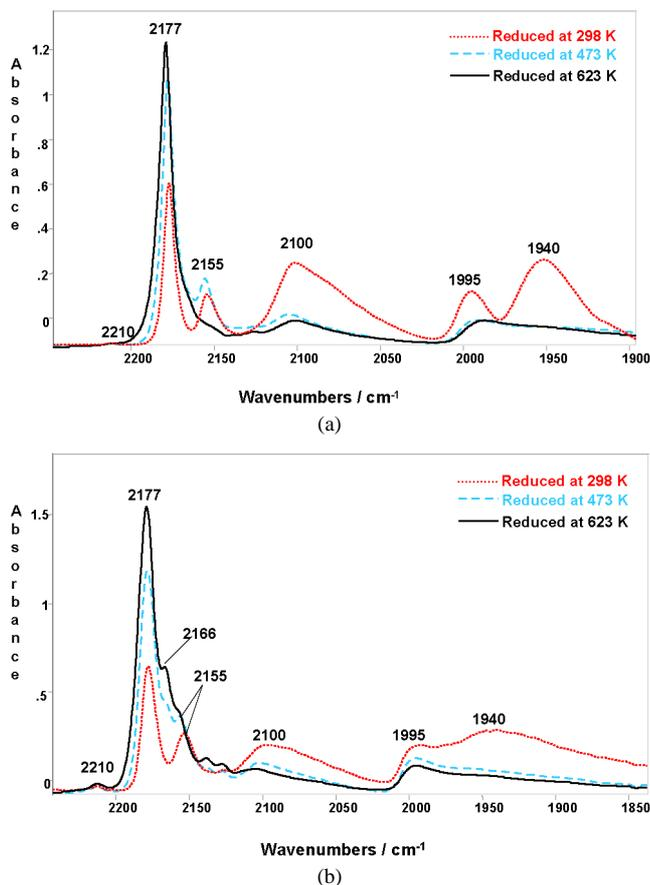
Fig. 3. FTIR spectra following exposure of samples (a) Pd\_P25; and (b) Pd\_Ana to 50 mbar of CO at 100 K, for samples reduced at different temperatures.
