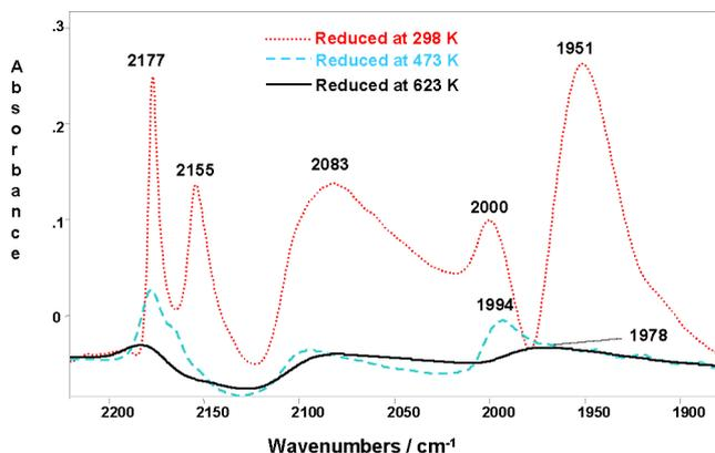
Fig. 4. Modifications to CO adsorption following exposure of the catalyst to 10 mbar of O<sub>2</sub>. The spectra presented are the difference between the spectrum of CO adsorption before and after dosing of O<sub>2</sub>. FTIR collected at 100 K and adsorption carried out with 50 mbar of CO on Pd\_P25.
