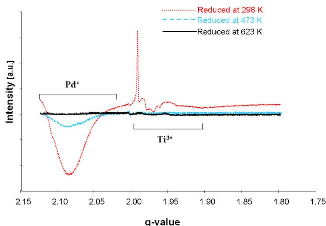
Fig. 2. EPR of Pd\_Ana, collected at 77 K, reduced at different temperatures with 1 mbar of H<sub>2</sub> and evacuated before cooling.
