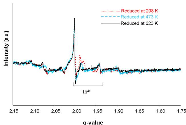
Fig. 1. EPR of Pd\_P25 collected at 77 K, reduced at different temperature and cooled in 1 mbar of H<sub>2</sub>.
