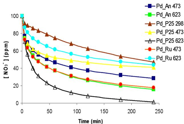
Fig. 6. Nitrates conversion profiles as a function of time for all catalysts.
