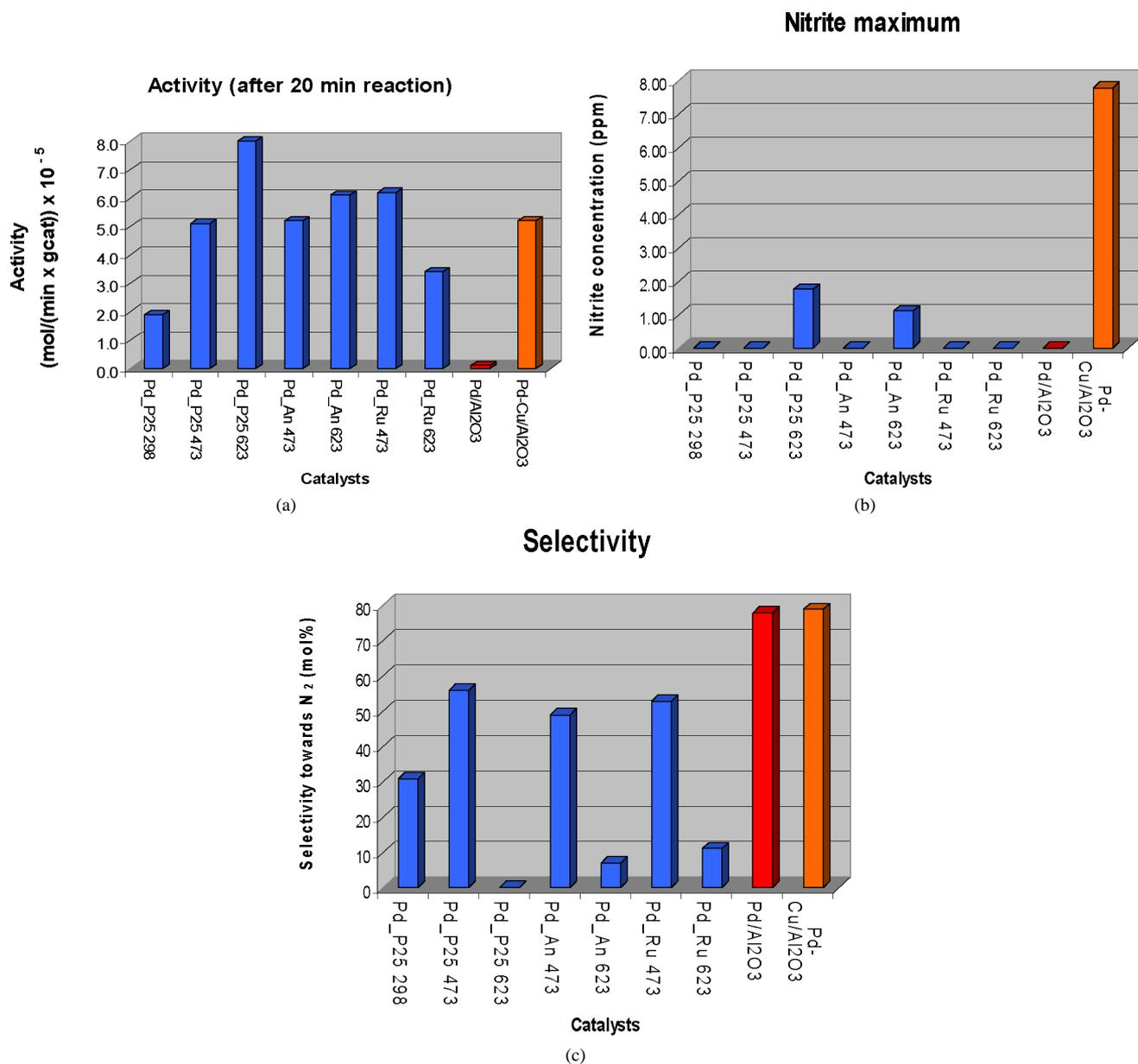
Fig. 5. Catalytic performances of the catalysts: (a) activity (after 20 min reaction); (b) maximum concentration of  $\text{NO}_2^-$ ; (c) selectivity to  $\text{N}_2$ .
