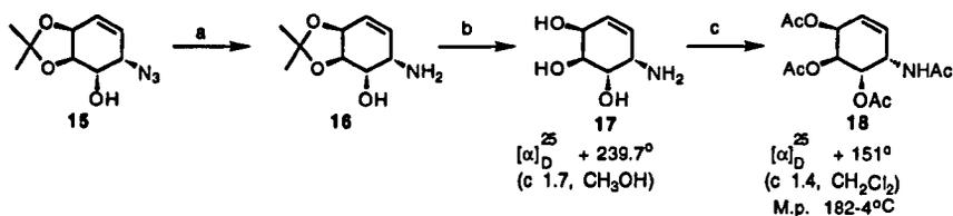
a) (CH<sub>3</sub>)<sub>3</sub>P, THF, H<sub>2</sub>O, 94%. b) 2N HCl, H<sub>2</sub>O, THF, 88%. c) Ac<sub>2</sub>O, C<sub>2</sub>H<sub>5</sub>N, 70%
