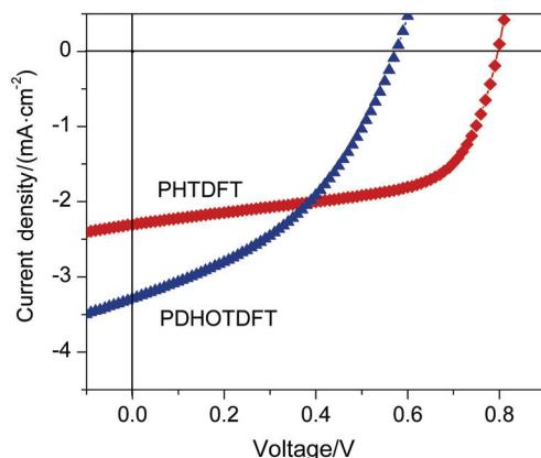
**Figure 3**  $J$ - $V$  curves of the PSC devices based on PHTDFT and PDHOTDFT under illumination of AM 1.5G, 100 mW/cm<sup>2</sup>.
