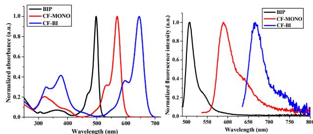
**Figure 2. Normalized absorbance and emission spectra of Bodipy fluorophores in acetonitrile**
