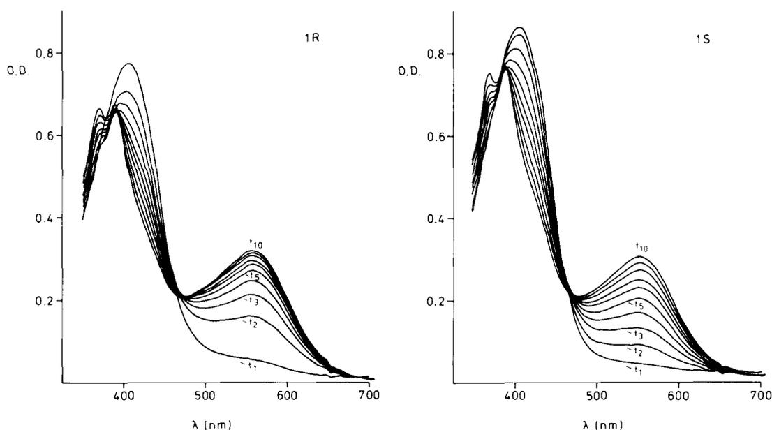
Figure 8. Time-dependent absorption spectra of reaction of excess of (all-*E*)-(R)- and (all-*E*)-(S)-5-demethyl-8,16-methanoretinal with bO (concn.  $7.5 \cdot 10^{-6}$  M).  $\lambda_{\text{max}}[\text{bR}(\mathbf{1a})] = \lambda_{\text{max}}[\text{bR}(\mathbf{1b})] = 552$  nm.  $t_1 = 11''$ ,  $t_2 = 1'.24''$ ,  $t_3 = 2'.37''$ ,  $t_5 = 6'.11''$ ,  $t_{10} = 19'.11''$ .
