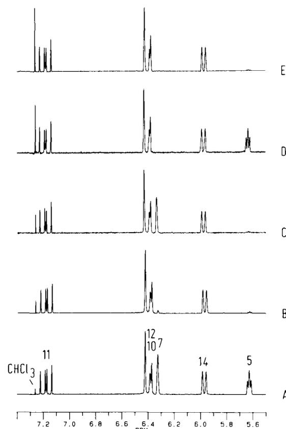
Figure 7. Vinyl region of 300-MHz  $^1\text{H}$  NMR spectrum of all-E isomers of **1** (A), **1c** (B), **1d** (C), **1e** (D), **1f** (E).
