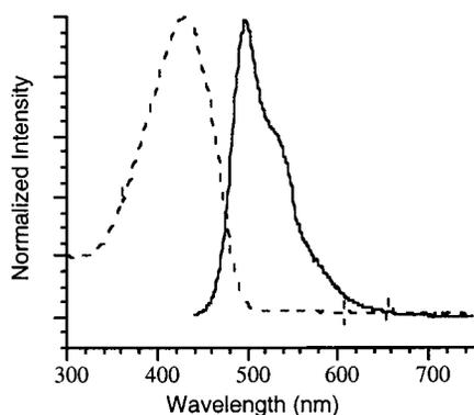
**Figure 2.** Absorption (---) and emission (—) spectra of **7b** ( $M_n = 4700$ ).
