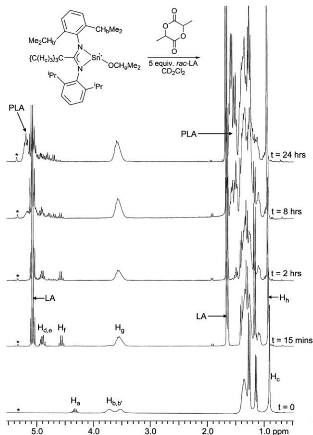
**Fig. 8** <sup>1</sup>H NMR spectra of the reaction between **3** and 5 equivalents *rac*-LA ( $\text{CD}_2\text{Cl}_2$ , 298K, 250 MHz; \* =  $\text{CHDCl}_2$ ). Spectrum shown at  $t = 0$  was recorded prior to monomer addition.
