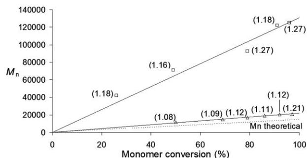
**Fig. 9** A plot of  $M_n$  vs. monomer conversion for the polymerisation of *rac*-LA using complexes **4** ( $\Delta$ ) and **5** ( $\square$ ) as the initiator (60 °C; toluene  $[\text{LA}]_0 : [\mathbf{4}] = 100$ ;  $[\text{LA}]_0 : [\mathbf{5}] = 100$ ; polydispersities given in parentheses).
