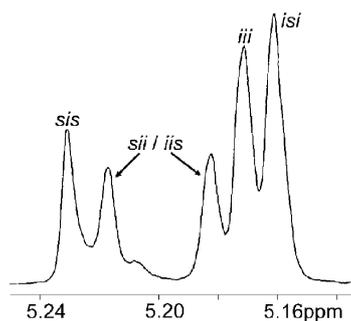
**Fig. 10** The methine region of the  $^1\text{H}$  decoupled NMR spectrum (298 K, 400 MHz,  $\text{CDCl}_3$ ) of PLA prepared using complex **3** at 60 °C in toluene (*i* = isotactic, *s* = syndiotactic dyads).
