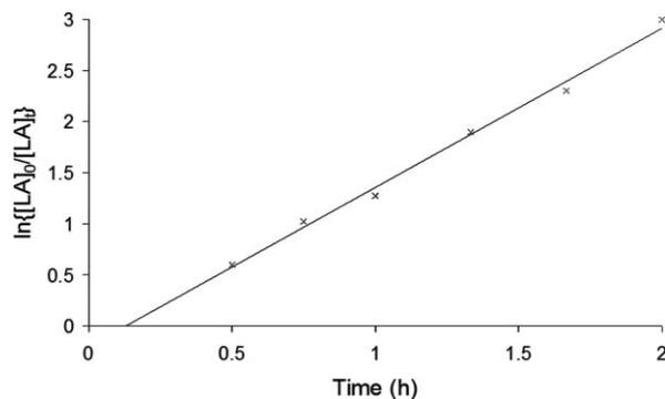
**Fig. 7** A plot of  $\ln\{[LA]_0/[LA]_t\}$  vs. time for the polymerisation of *rac*-LA using complex **3** as the initiator (60 °C; toluene; [LA]<sub>0</sub> = 0.28 M; [3] = 0.0014 M; [LA]<sub>0</sub> : [3] = 200).
