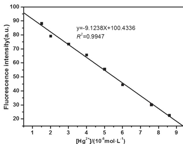
Fig. 4 Fluorescence intensity of **4** as a function of concentration of  $\text{Hg}^{2+}$  ( $0.8$ – $8.4 \mu\text{mol L}^{-1}$ ).
