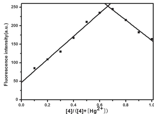
Fig. 5 Job's plot of **4** and  $\text{Hg}^{2+}$  ( $[\text{4}] + [\text{Hg}^{2+}] = 10 \text{mmol L}^{-1}$ ).
