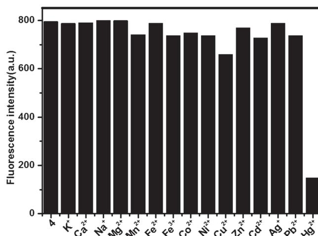
**Fig. 1** The effect of metal ions (10 μM) on the fluorescent properties of probe **4** (10 μM) in 100 mM Tris-HCl buffer (pH 7.4) (H<sub>2</sub>O:EtOH=9:1, v/v) with an excitation at 368 nm. The samples were incubated for 10 min at room temperature prior to measurements.
