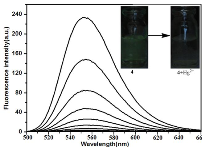
Fig. 3 The emission intensity of **4** ( $10 \mu\text{mol L}^{-1}$ ) changes with increasing concentrations of  $\text{Hg}^{2+}$  ( $0$ – $30 \mu\text{mol L}^{-1}$ ), the inset shows photograph of **4** ( $10 \mu\text{mol L}^{-1}$ ) in the absence and presence of  $\text{Hg}^{2+}$  under UV light (365 nm).
