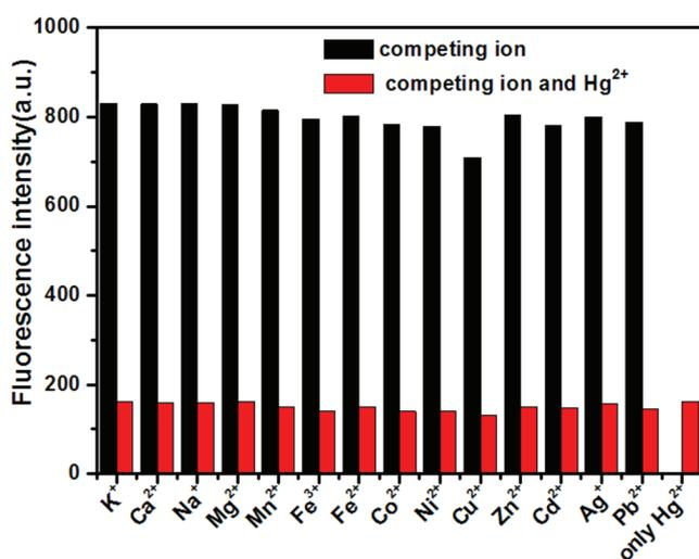
Fig. 2 The effect of  $\text{Hg}^{2+}$  on **4** ( $10 \mu\text{mol L}^{-1}$ ) in the presence of different metal ions ( $100 \mu\text{mol L}^{-1}$ ).
