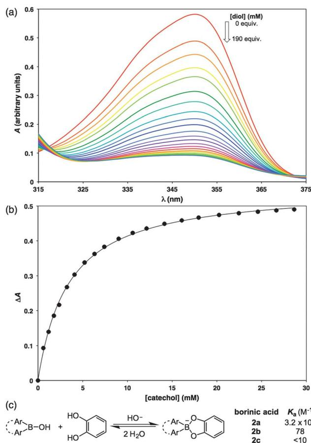
**Fig. 4** (a) Overlay of absorption spectra of **2a** (0.15 mM) upon addition of catechol in a 10 mM HEPES (3 : 1 CH<sub>3</sub>OH : H<sub>2</sub>O), pH 7.4 solution. (b) Data from (a) fitted to a 1 : 1 binding isotherm. (c) Average *K*<sub>a</sub> of duplicate trials (±20%) for borinic acids **2a–c**.
