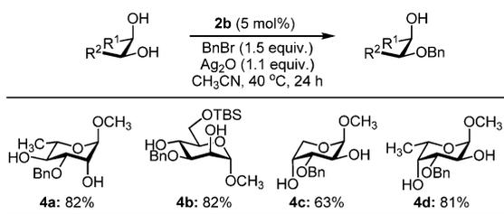
**Scheme 3** Selective monobenylation of pyranoside substrates catalyzed by **2b**.
