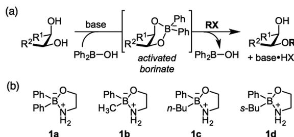
**Scheme 1** (a) Borinic acid catalyzed diol activation; and (b) structures of borinic ester precatalysts **1a–d**.
