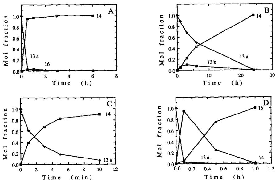
Fig. 6. Reductive cleavage of methyl 2,3,4-tri-*O*-methyl-6-*O*-propionyl- $\alpha$ -D-glucopyranoside (**13a**) in the presence of A,  $\text{Me}_3\text{SiOSO}_2\text{CF}_3$ ; B,  $\text{BF}_3 \cdot \text{Et}_2\text{O}$ ; and C and D,  $\text{Me}_3\text{SiOSO}_2\text{Me}-\text{BF}_3 \cdot \text{Et}_2\text{O}$ .
