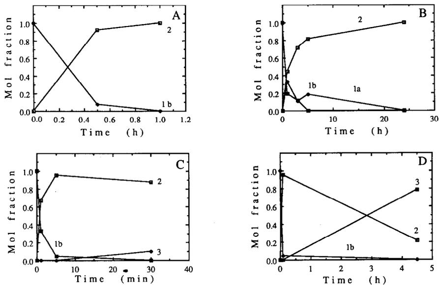
Fig. 1. Reductive cleavage of methyl 3,4,6-tri-*O*-methyl-2-*O*-propionyl-β-D-glucopyranoside (**1b**) in the presence of A, Me<sub>3</sub>SiOSO<sub>2</sub>CF<sub>3</sub>; B, BF<sub>3</sub>·Et<sub>2</sub>O; and C and D, Me<sub>3</sub>SiOSO<sub>2</sub>Me-BF<sub>3</sub>·Et<sub>2</sub>O.
