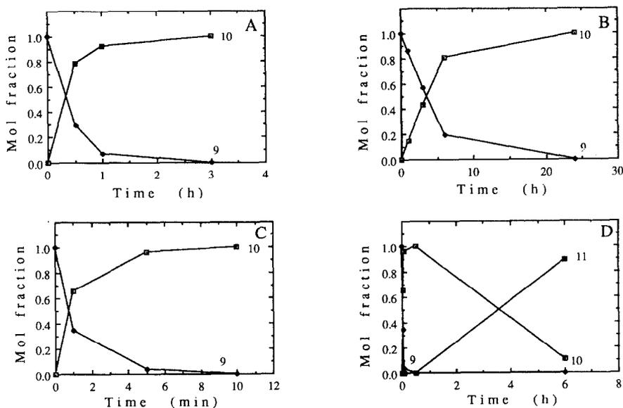
Fig. 5. Reductive cleavage of methyl 2,3,6-tri-*O*-methyl-4-*O*-propionyl- $\alpha$ -D-glucopyranoside (9) in the presence of A,  $\text{Me}_3\text{SiOSO}_2\text{CF}_3$ ; B,  $\text{BF}_3 \cdot \text{Et}_2\text{O}$ ; and C and D,  $\text{Me}_3\text{SiOSO}_2\text{Me}-\text{BF}_3 \cdot \text{Et}_2\text{O}$ .
