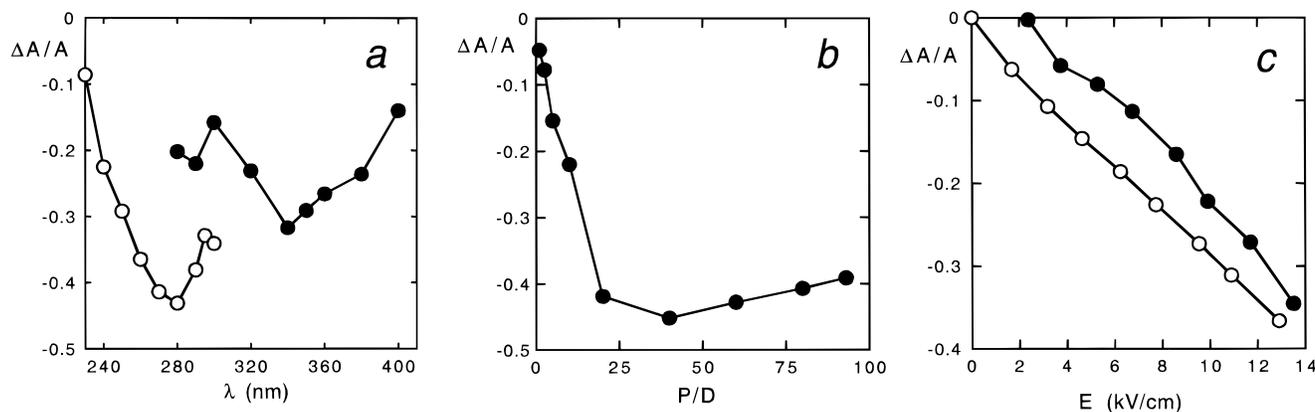
**Figure 3.** Dependence of the reduced dichroism  $\Delta A/A$  on (a) wavelength, (b) the DNA-phosphate to drug ratio (P/D), and (c) electric field strength for compound **1**-DNA complex (J) and for DNA alone (E). Conditions: (a) P/D = 20, 12.5 kV/cm, (b) 340 nm, 12.5 kV/cm, (c) 340 nm for **1**, 260 nm for DNA, P/D = 20 in 1 mM sodium cacodylate buffer, pH 6.5.
