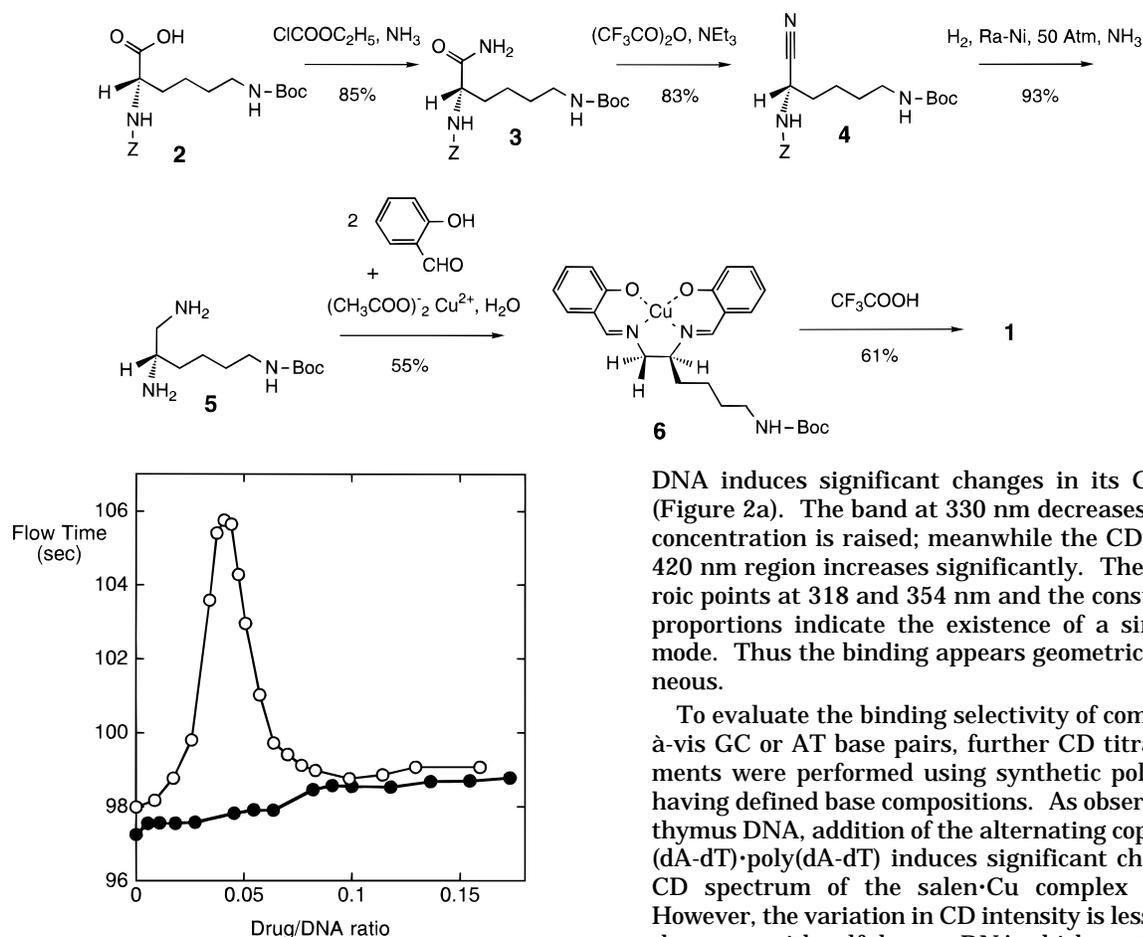
**Figure 1.** Viscometric titrations of pUC12 closed circular duplex DNA with compound **1** (J) and ethidium bromide (E). The flow time is plotted as a function of the molar ratio of drug added per DNA nucleotide.
