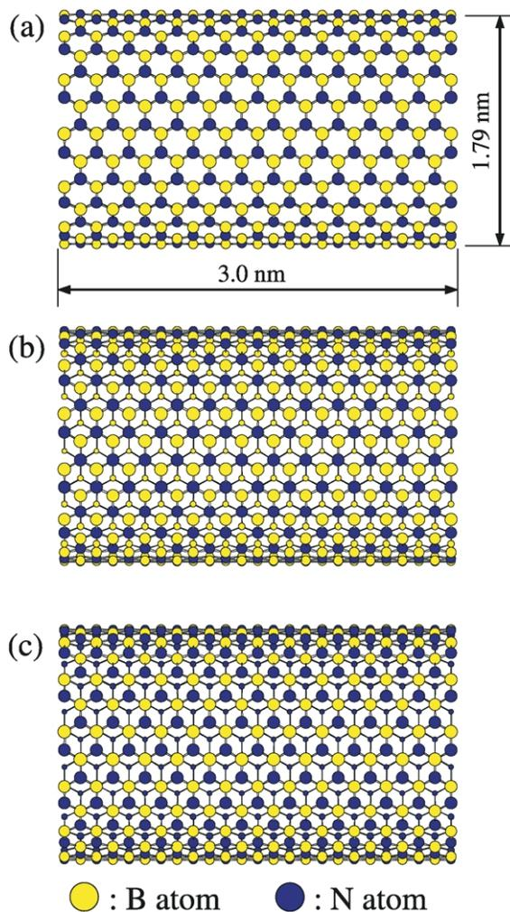
Fig. 2. Proposed structure models of single-walled BN nanotubes.
