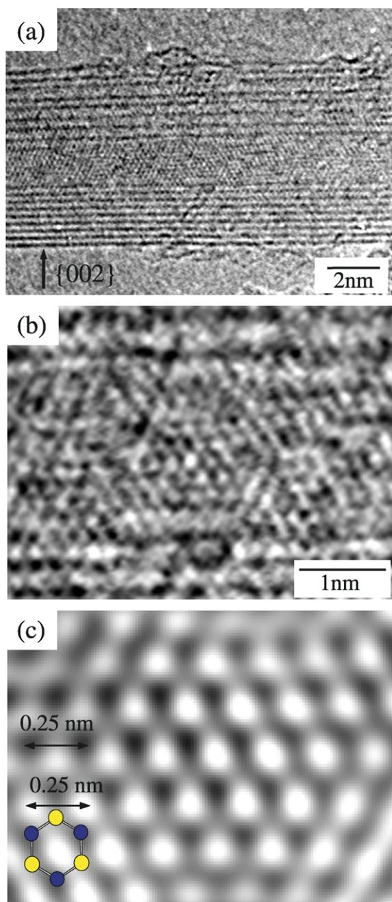
Fig. 1. (a) HREM image, (b) enlarged image and (c) processed image of BN nanotube produced from  $YB_6$  powder.
