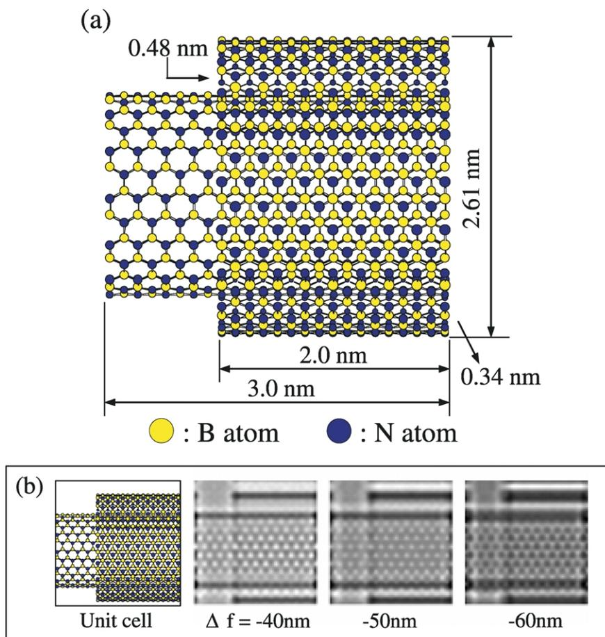
Fig. 4. (a) Proposed structure model of double-walled BN nanotubes. (b) Calculated HREM images of (a) as a function of defocus values.
