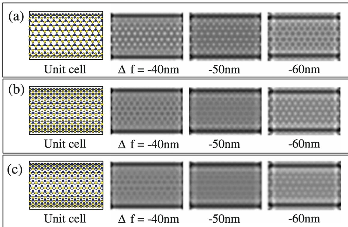
Fig. 3. (a)–(c) Calculated HREM images of Fig. 2(a)–(c), respectively.
