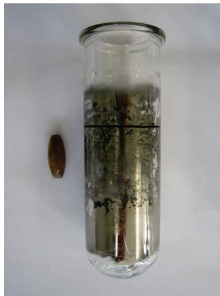
Figure 4. Pd-coated reaction vessel and stirrer bar.
