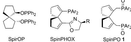
**Scheme 1.** Structures of SpirOP, SpinPHOX, and SpinPO (1).
