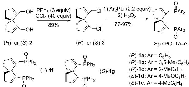
**Scheme 2.** Preparation of enantiopure phosphine oxides **1a–e**, and the structures of **1f–g**.
