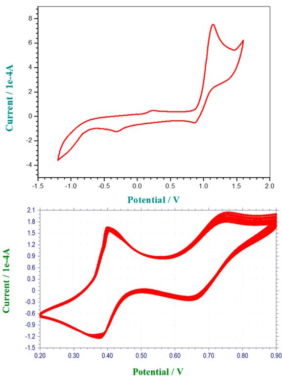
**Figure 3.** Cyclic voltammogram of **12** (top) and **24** (bottom, 40 cycles) recorded in  $CH_3CN$  ( $1 \times 10^{-3}$  M) containing  $TBAPF_6$  (0.1 M) as supporting electrolyte at a scan rate of 100 mV/s.
