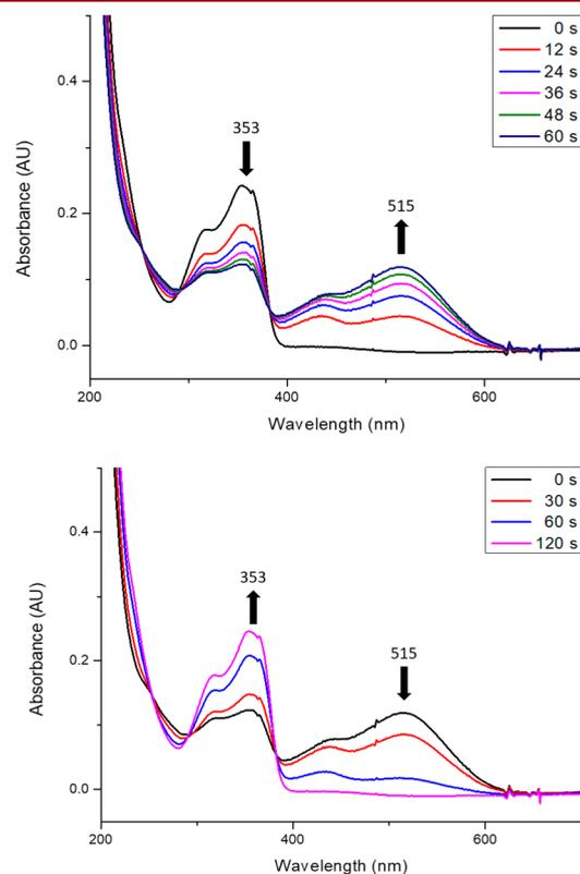
**Figure 4.** (Top) Spectroelectrochemical spectra of **24** in  $CH_3CN$  ( $5 \times 10^{-5}$  M) with 0.1 M  $TBAPF_6$  at an applied oxidation potential of 0.55 V (vs  $Ag/AgCl$ ). (Bottom) Spectroelectrochemical spectra of the oxidized **24** at an applied reduction potential of 0.20 V (vs  $Ag/AgCl$ ).
