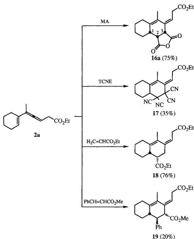
The assignment of the (*Z*) configuration to the exocyclic double bond and the determination of the relative configuration of the three centers of chirality of **16a** are based on the NMR data and an X-ray structure analysis<sup>[11a]</sup>. Thus,
