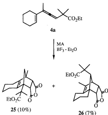
ingly, a variation of the Lewis acid does not affect the course of the reaction, but only the product yields; for example, with SbCl<sub>3</sub> 13% of **25** and 2% of **26** were isolated.
