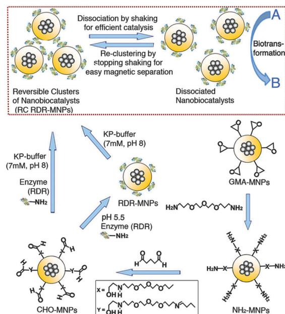
**Fig. 1** Synthesis and biocatalysis of reversibly clustered magnetic nanobiocatalysts.
