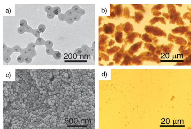
**Fig. 2** (a) TEM of CHO-MNPs. (b) Optical microscopy of RC RDR-MNPs. (c) FESEM of RC RDR-MNPs. (d) Optical microscopy of RC RDR-MNPs after shaking at 300 rpm and 30 °C for 2 min.
