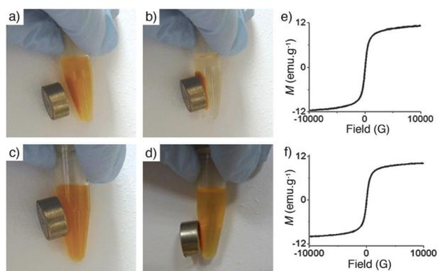
**Fig. 3** (a and b) Magnetic separation of RC RDR-MNPs: (a)  $t = 0$ , (b)  $t = 4$  s. (c and d) Magnetic separation of fine RDR-MNPs: (c)  $t = 0$ , (d)  $t = 20$  min. (e) VSM of RC RDR-MNPs. (f) VSM of fine RDR-MNPs.
