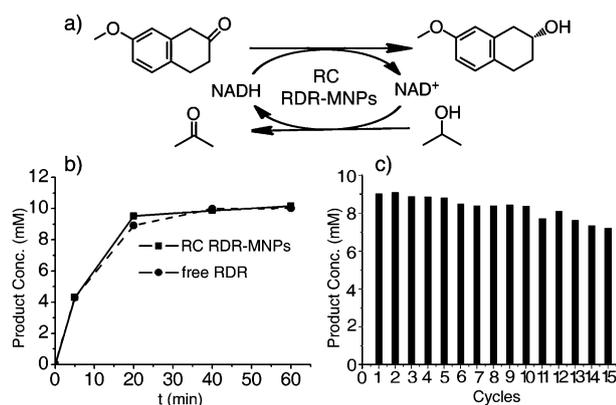
**Fig. 4** (a) Scheme of enantioselective bioreduction of 7-methoxy-2-tetralone with cofactor recycling. (b) Time course of the biotransformation at a pH of 8 with RC RDR-MNPs and free RDR, respectively. (c) Recycling of RC RDR-MNPs in the enantioselective bioreduction.
