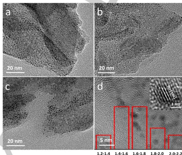
**Figure 2.** TEM images of (a) Ru/HAP, (b) Ru-Zn/HAP, (c) Ru-Zn-Cu(I)/HAP, (d) HRTEM and Ru particle size distribution of Ru-Zn-Cu(I)/HAP, the corresponding PSD histogram of the Ru NPs is given in the insert.
