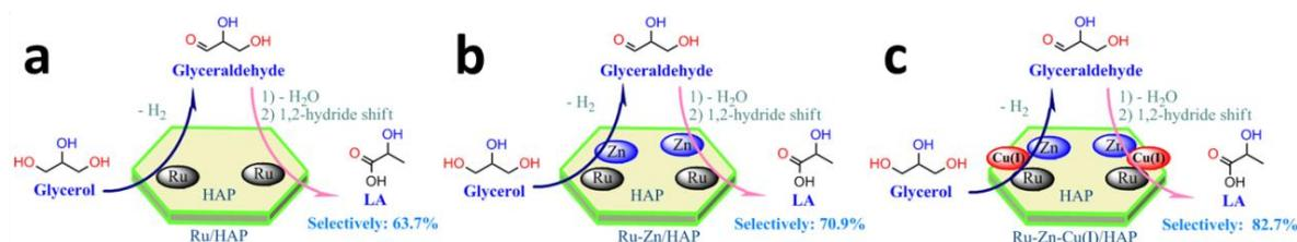
**Scheme 1.** Proposed reaction pathway for glycerol conversion over Ru/HAP (a), Ru-Zn/HAP (b), and Ru-Zn-Cu(I)/HAP (c).
