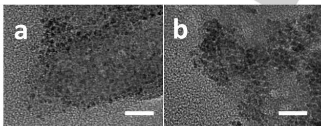
**Figure 6.** TEM images of fresh Ru-Zn-Cu(I)/HAP (a) and the Ru-Zn-Cu(I)/HAP after reused four times (b). The scar bar is 10 nm.
