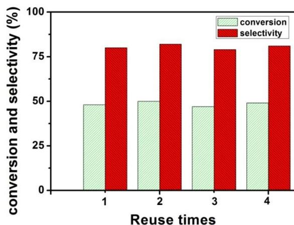
**Figure 5.** Reusability of the Ru-Zn-Cu(I)/HAP for glycerol conversion. Reaction conditions: 20 mg catalyst, 0.1 g glycerol, NaOH, 0.065 g, and 2 mL water, 6 h.
