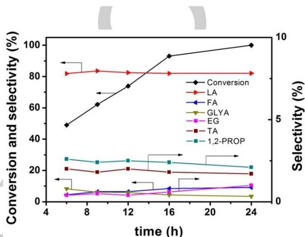
**Figure 4.** Time course of glycerol conversion over Ru-Zn-Cu(I)/HAP catalyst. Reaction conditions: 20 mg catalyst, 0.1 g glycerol, NaOH, 0.065g, and 2 mL water, 140 °C.
