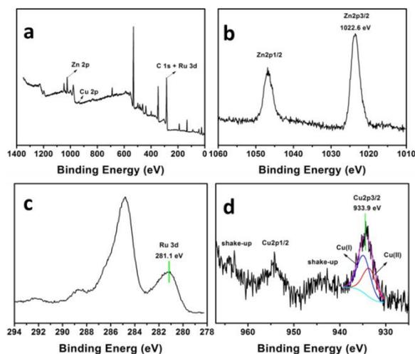
**Figure 3.** XPS spectra of the Ru-Zn-Cu(I)/HAP catalyst (a) full spectrum; (b) Zn 2p spectrum; (c) Ru 3d spectrum; (d) Cu 2p spectrum.
