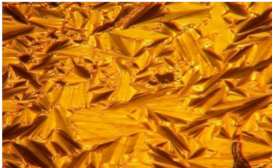
Fig. 3. Optical Texture of ligand (HL) at 175 °C
