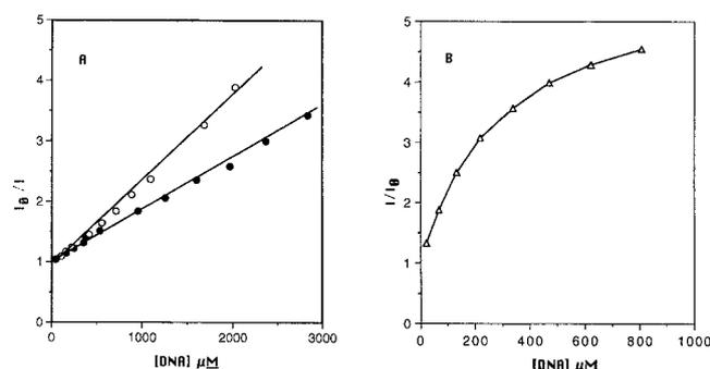
**Figure 3.** Fluorescence quenching (A) of furocoumarins **1a'** (open circles; 9.9  $\mu\text{M}$ ;  $\lambda_{\text{ex}} = 302$  nm and  $\lambda_{\text{em}} = 482$  nm) and **1b'** (filled circles; 10.5  $\mu\text{M}$ ;  $\lambda_{\text{ex}} = 304$  and  $\lambda_{\text{em}} = 502$  nm) and fluorescence enhancement (B) of furocoumarin **2a** (open triangles; 9.5  $\mu\text{M}$ ;  $\lambda_{\text{ex}} = 336$  and  $\lambda_{\text{em}} = 511$  nm) as a function of DNA concentration.
