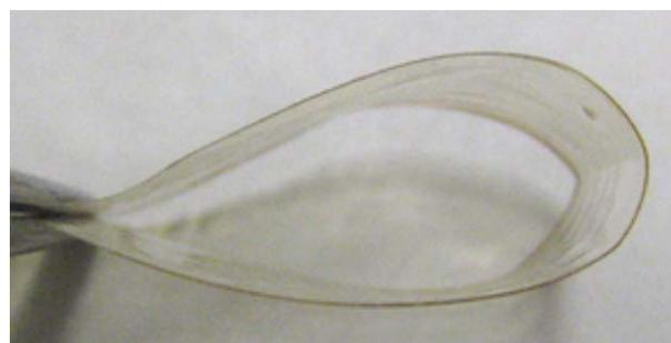
FIGURE 8 Bent film of network polymer (**N-PEK5** with 1 mol % TsOH). [Color figure can be viewed in the online issue, which is available at [wileyonlinelibrary.com](http://wileyonlinelibrary.com).]
