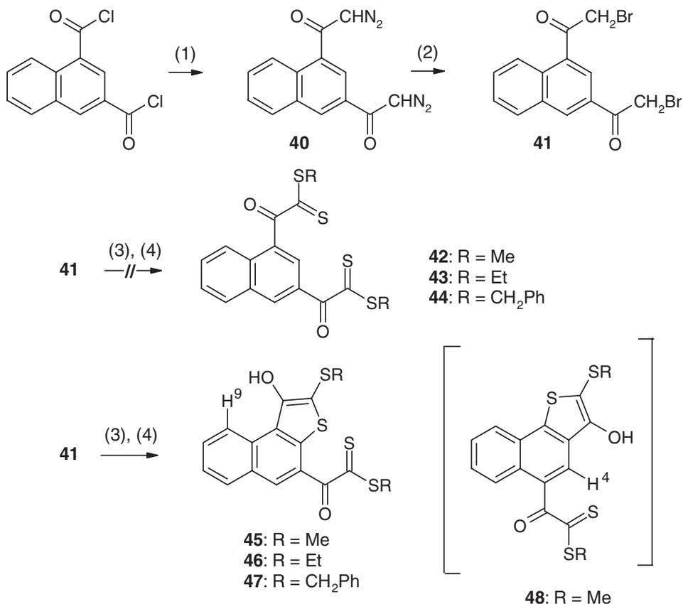
**Scheme 7** (1): CH<sub>2</sub>N<sub>2</sub>; (2): HBr; (3): S<sub>8</sub>, NEt<sub>3</sub>, DMF; (4) RI.
