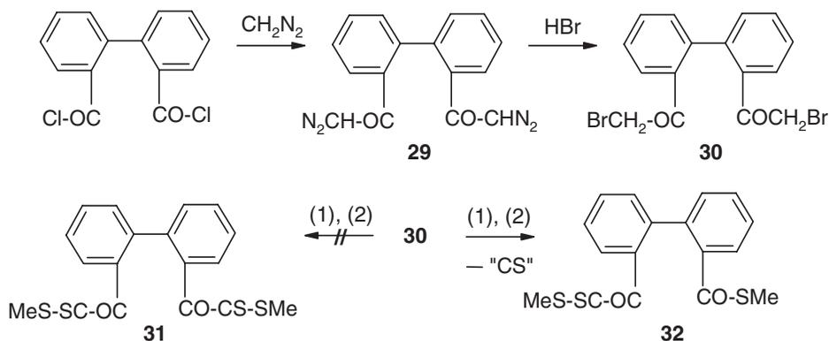
Scheme 5 (1): S<sub>8</sub>, NEt<sub>3</sub>, DMF; (2): Mel.
