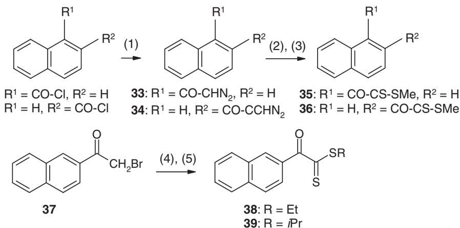
Scheme 6 (1): CH<sub>2</sub>N<sub>2</sub>; (2): S<sub>8</sub>, NEt<sub>3</sub>, CaCl<sub>2</sub>, DMF; (3): Mel; (4) S<sub>8</sub>, NEt<sub>3</sub>, DMF; (5): RI.
