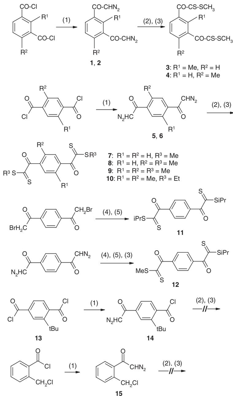
**Scheme 1** (1): CH<sub>2</sub>N<sub>2</sub>; (2): S<sub>8</sub>, NEt<sub>3</sub>, CaCl<sub>2</sub>, DMF; (3): MeI, (4): S<sub>8</sub>, NEt<sub>3</sub>, DMF; (5): *i*PrI.
